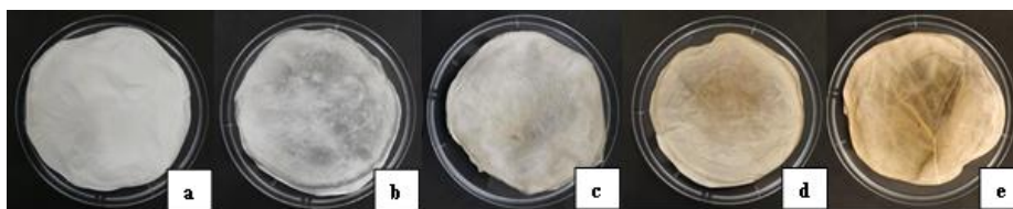
Figure 2. Purified BC sheets with various NaOH concentration (a) 0%, (b) 0.5%, (c) 1.0%, (d) 2.0% and (e) 3.0% w/v, NaOH
