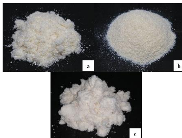
Figure 4. Appearance of BC powder (a) commercial BCP, (b) BCP-M1 and (c) BCP-M2
