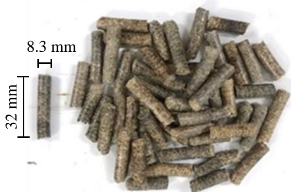
Figure 2. Biomass pellets from giant sensitive plant
