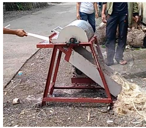
Figure 2. Actual field testing of the abaca deco machine
