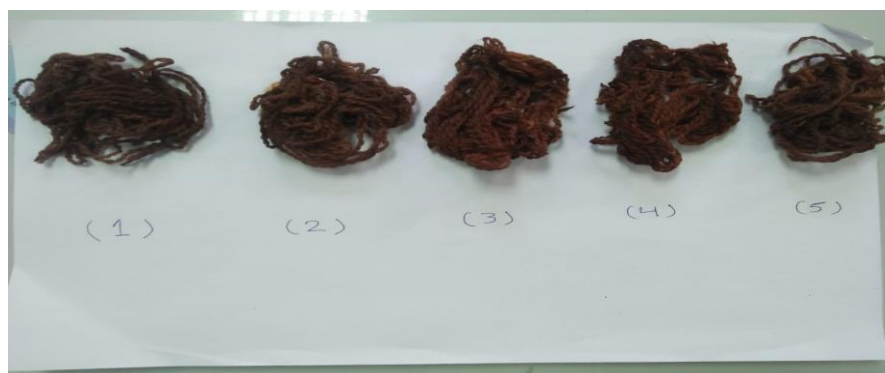
Figure 1. Samples dyed with the investigated at different time intervals (1-5) min. by microwave
