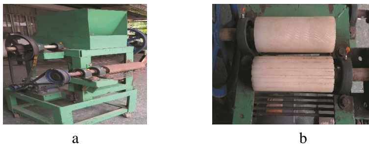
Figure 1. Groundnut shelling unit, a = testing machine and b = shelling roller
