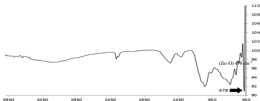
**Figure 3.2.** FTIR spectra of the synthesized ZnO nanoparticles.
