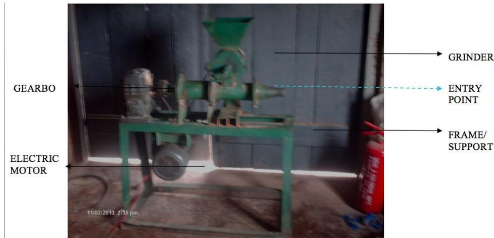
**Plate 2:** The Combined Grinding and Pelletizing Machine
