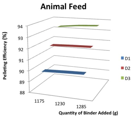
**Fig. 2c.** Surface Response of Pelleting Efficiency to Animal Feed Quantity and Pellets Diameter
