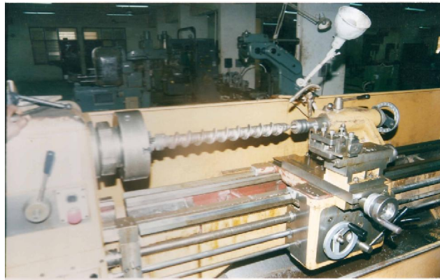
Fig. 1 Lathe machining of Screw Expellant Shaft.
